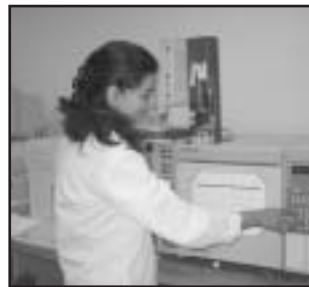
Reem Musleh (MSU) uses gas chromatography to measure the volatile organic acids in leachate samples.
