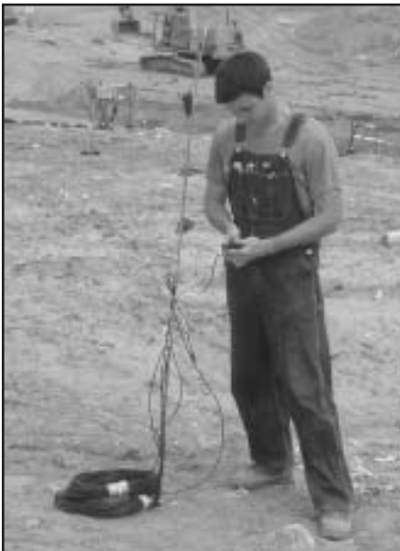
Seth Maher (MSU) reads moisture probes installed in the bioreactor landfill cap.
